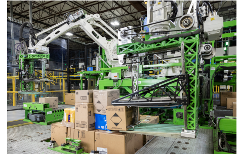
Symbotic robotic case-picking system building mixed-SKU pallets
