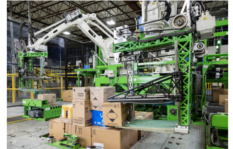
Symbotic robotic case-picking system building mixed-SKU pallets
